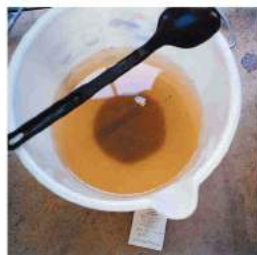
Floc formation after PUR addition
