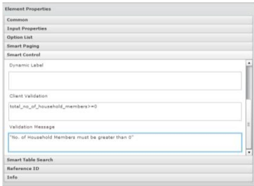
The screenshot shows the 'Element Properties' dialog box with the 'Client Validation' field containing the expression `total_no_of_household_members >= 0` and the 'Validation Message' field containing the text `"No. of Household Members must be greater than 0"`.
