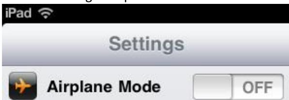
5. **Wireless connectivity** consumes much of the device battery power. Even though there may not be wireless connectivity in the area where the people using the devices will operate, the device will constantly be searching for a connection, and the batter will be drained faster.
