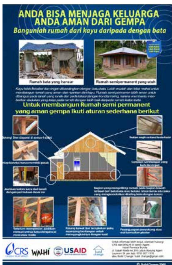
Illustrated technical guide for transitional shelter construction in Padang, West Sumatra, Indonesia, 2009
